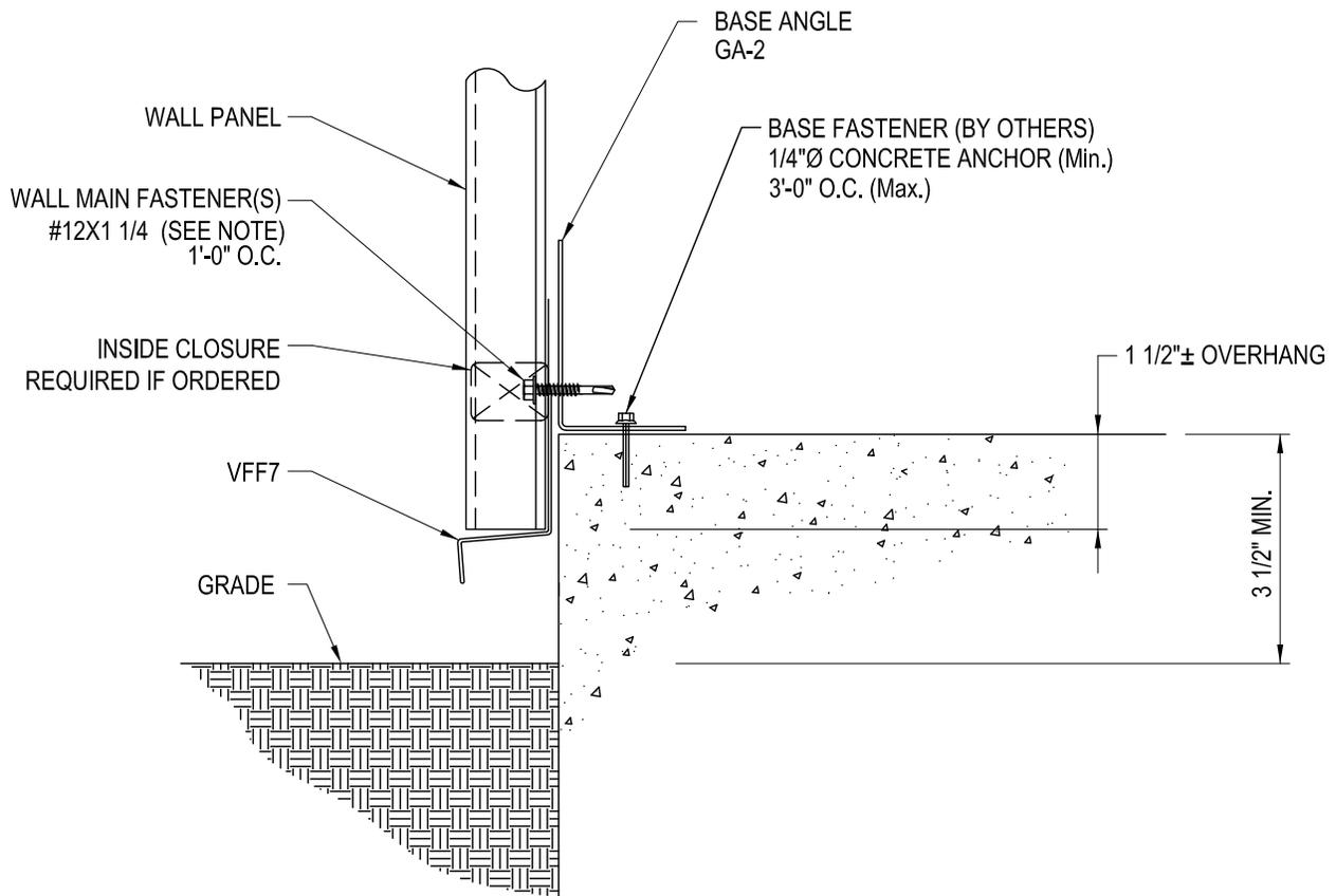
NOTE: #12X2 FASTENERS w/ 6" INSULATION.
