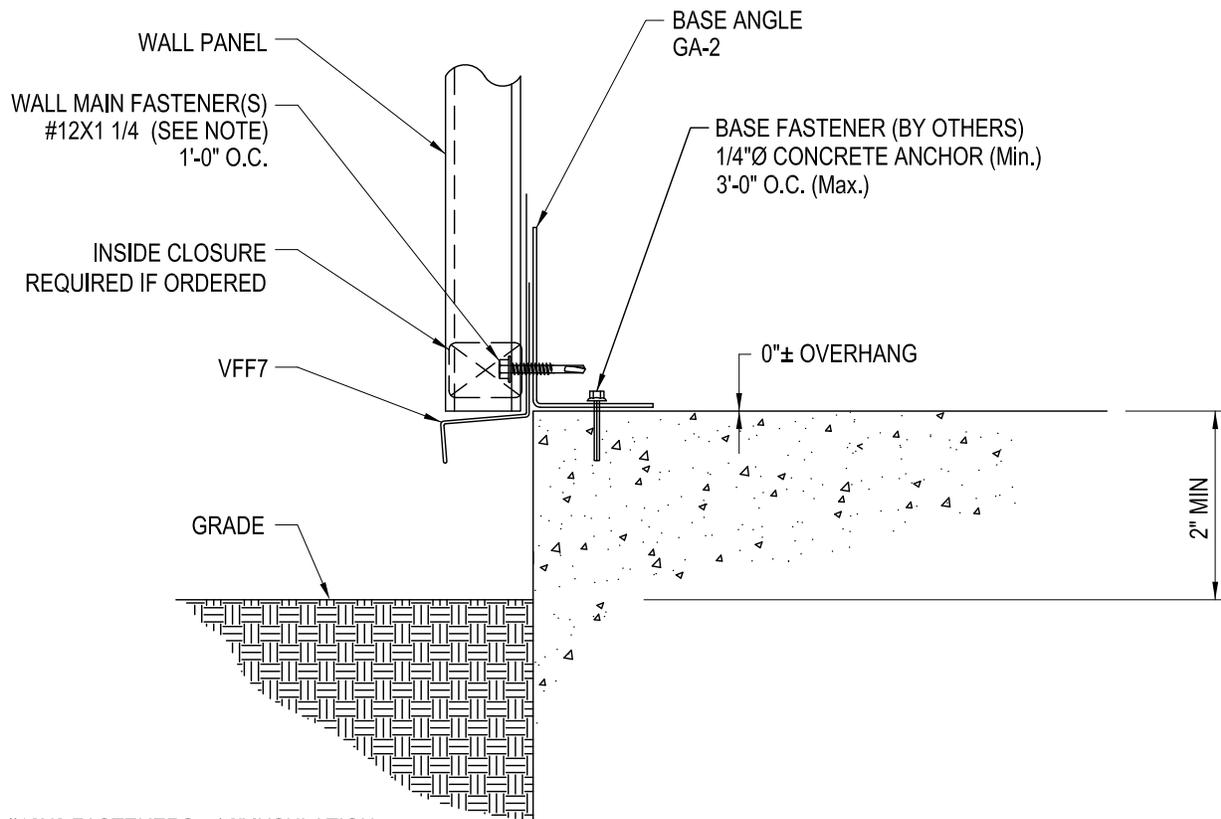
NOTE: #12X2 FASTENERS w/ 6" INSULATION.
