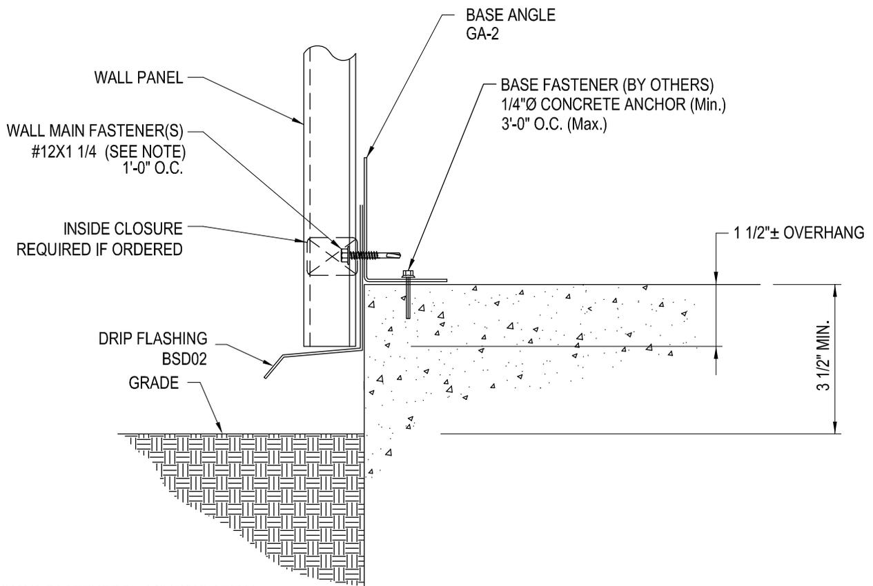
NOTE: #12X2 FASTENERS w/ 6" INSULATION.
