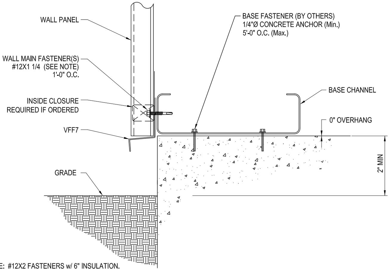
**SECTION AT BASE CHANNEL (WALL PANEL FLUSH TO FLOOR)**
