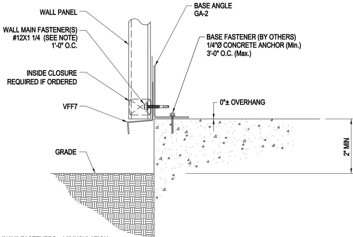
NOTE: #12X2 FASTENERS w/ 6" INSULATION.
