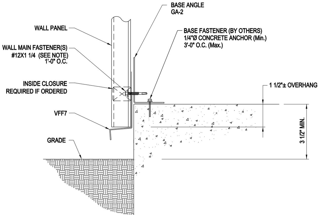
NOTE: #12X2 FASTENERS w/ 6" INSULATION.
