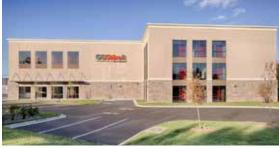
A total of five buildings, this self storage facility is fully climate controlled. Building one is L-shaped, with two full mezzanines, elevators, and surrounding parapet walls. The exteriors are a combination of brick, metal panel, and EIFS.
