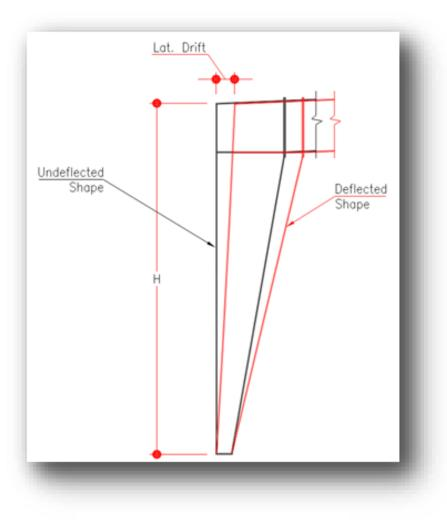
Figure 1 - Frame Lateral Drift (sidesway)
