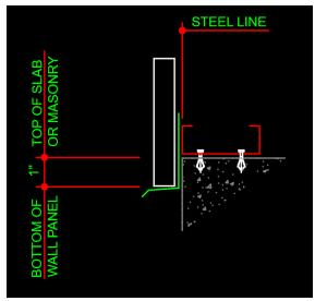
Gutter Extension Trim Options on the On-Slope Gutter
